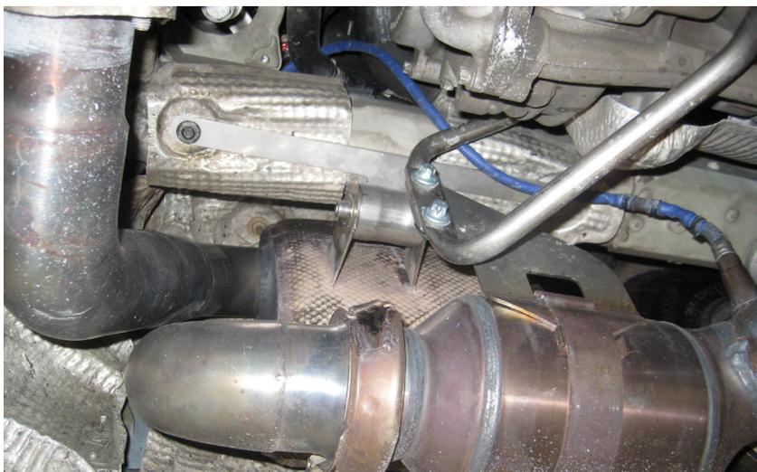
Additionally the pre silencers are equipped with a service opening, which can be used to refill the pre silencer with insulating material.
