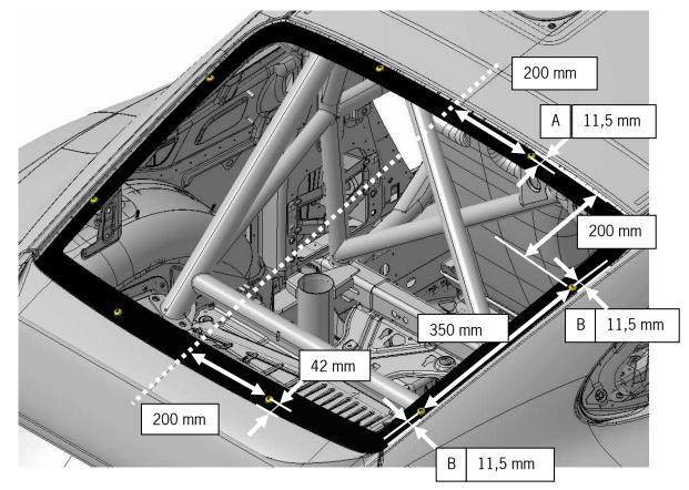
Detail view A and B (Distance between bore center and edge of window) for top and side bores.
