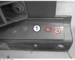
4.15.1.30 Remove adhesive residue from support (blue hatched area)
