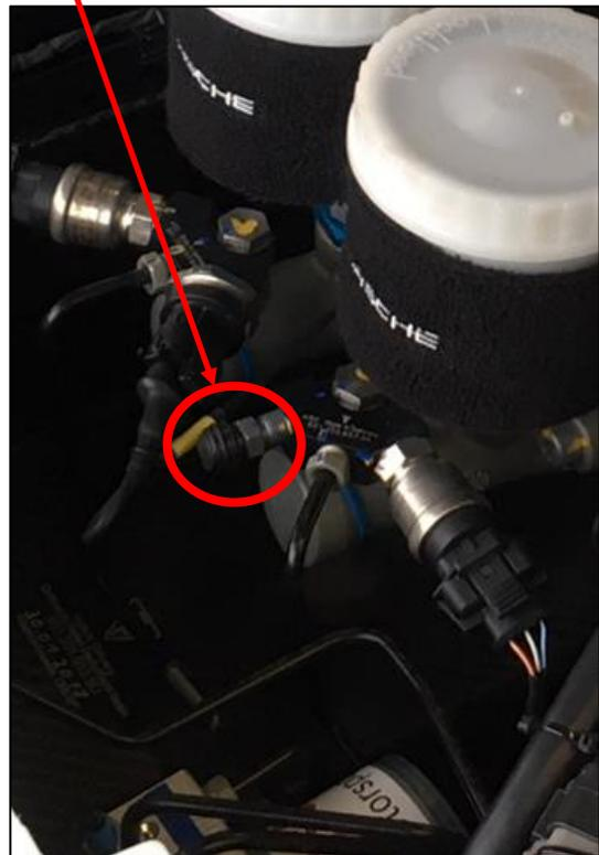
Porsche Motorsport recommends inspecting the blanking plug for leaks on any of the aforementioned vehicles equipped with an ABS kit from Manthey – Racing before the next operation. The blanking plug is attached to the brake master cylinder (BMC) for the rear axle (left in the direction of travel), and is shown circled in red in the images below. Any form of leaks or poor sealing is to be promptly addressed to Manthey Racing at [aftersales@manthey-racing.de](mailto:aftersales@manthey-racing.de).
