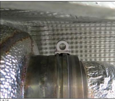
Tighten the two screws oft the ball clamp by hand. The front muffler must be movable (Figure 1.9.15)
