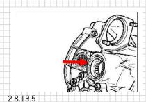
Drive out the differential cylinder roll bearing (Figure 2.8.13.5) with removal tool HAZET 788-70 (3) and panel puller
