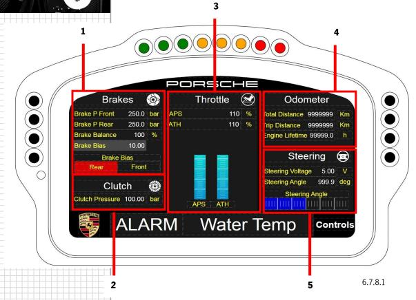
The "Control" page (Figure 6.7.8.1) of the display shows all the important information about the pedals and steering wheel. This means that the brake pressures as well as the position/function of the gas pedal and the electronic throttle valve can be checked.
