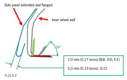
Figure 4.15.3 shows the reference measurement points. The reference measurement Y (image 4.15.5.4) corresponds to the measurement from the outer wheel arch flange edge to the wheel arch inner wall.
