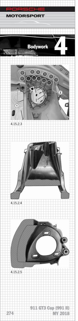
Drill the marked rivets using a solid carbide drill ( $\emptyset$  6.7 mm (0.26 inches)) from behind (if accessible) until they can be knocked out using a drift punch ( $\emptyset$  6.0 mm (0.24 inches)).
