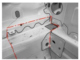
4.15.1.17 Cut of body front section, red dashed line, do not damage support in rear area.
