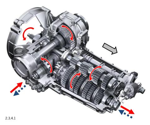
The torque is transmitted from the engine through the connecting shaft and drive shaft to the gearbox and then through the corresponding gear ratio from the drive shaft to the pinion shaft. The direction of the torque/speed is changed from the longitudinal to transverse direction by means of the cross shaft with constant ratio. The final drive ratio transmits the torque through the limited-slip differential to the axle flanges and finally through the axle shafts to the driving wheels.
