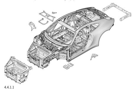
The new 911 GT3 Cup (991 II) has a body in aluminum-steel hybrid construction. The idea behind this concept of intelligent lightweight construction is to use the "right material in the right place". This means:
