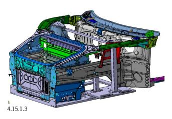
The chassis jig is required to check the mounting points for dimensional accuracy and tolerance. This jig is also required to adjust and fix in position a new front chassis section before all the rivets are inserted and seated.
