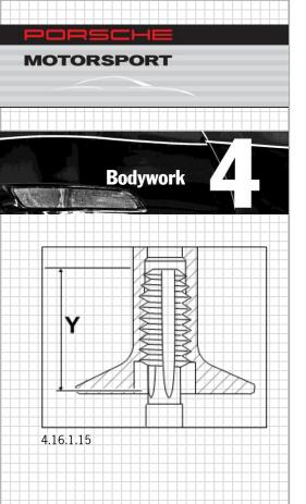
Cut the thread to the dimension (Y) with a cutting tool
