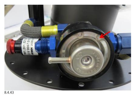
Tank plate connection layout
