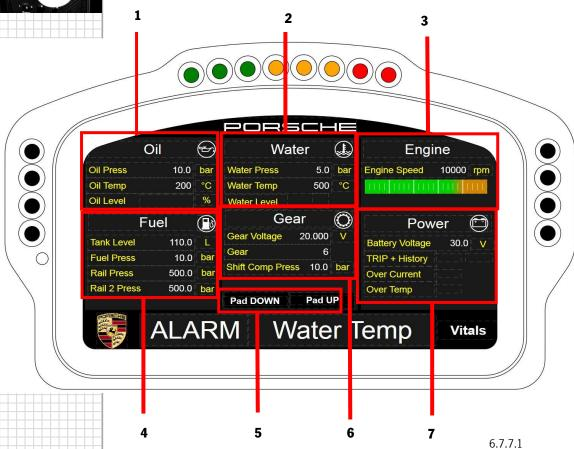
The "Vitals" page (Figure 6.7.7.1) provides an overview of the vital functions of the engine and vehicle. All the important channels are shown on one page here. The views and values are fixed on this page and cannot be changed.
