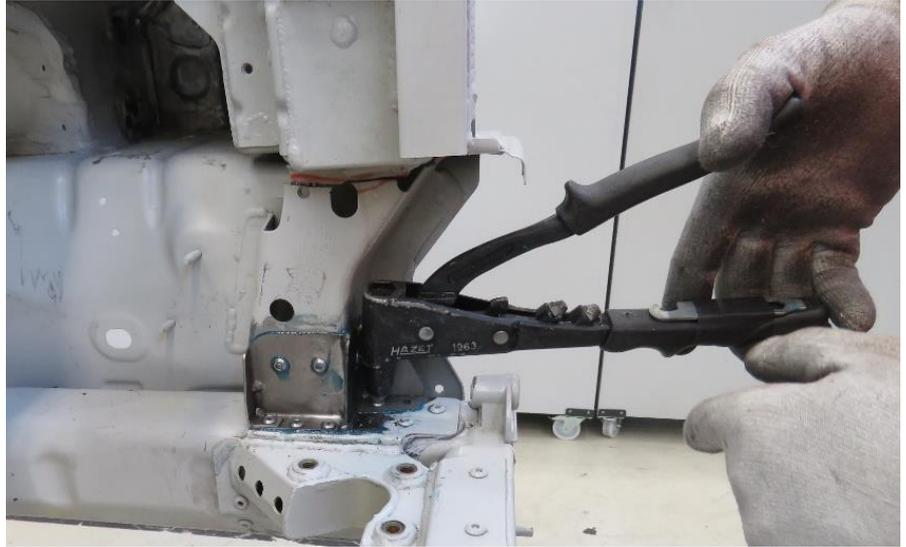
6. Fit the lower six rivets 4.8x6 & 7.5 using the hand riveter.
