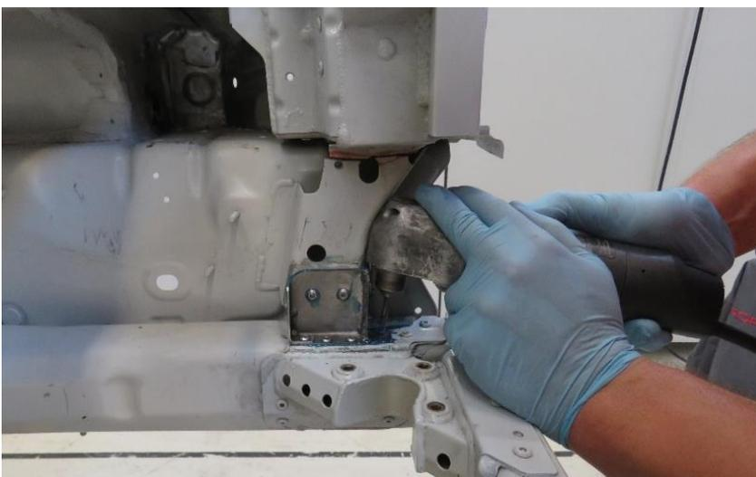
5. Bore out the lower rearward rivets holes using a 5 mm drill bit (use a drill bit with a length of 60 mm).
