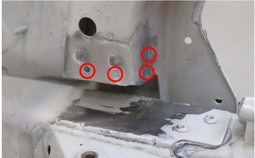
6. Use a punch / drift to knock out the rivet bodies (red circles).
