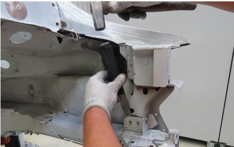
4. Remove the mounting using a hammer and chisel.
