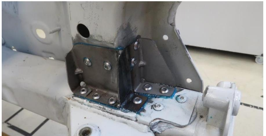
7. Remove any residual adhesive and clean the components.
